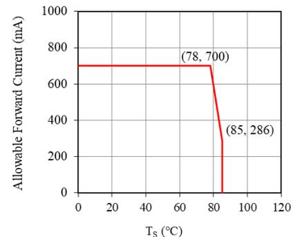
Figure 1.  $T_S$  vs Allowable Forward Current
