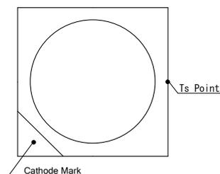
Figure 2.  $T_S$  Measurement point
