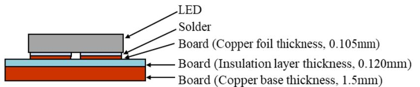
Figure 3. Structure of the board + LED
